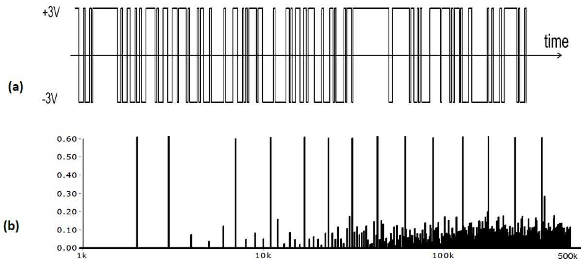
**Figure 1** Example of a spectrally sparse multi-frequency binary waveform (a) with known spectral content (b), which is used as excitation signal.
