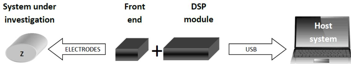
**Figure 2** Quadra platform implementation with stand-alone modules and host PC.
